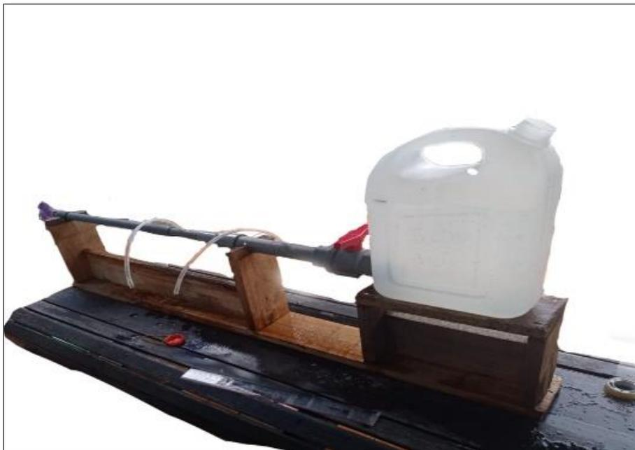
**Gambar 4.** Alat Venturimeter tanpa manometer
